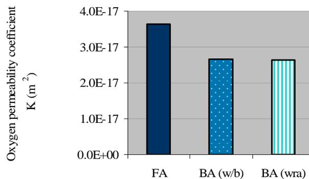
**Fig. 3.3** Oxygen permeability of FA and BA concretes
