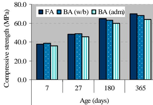
**Fig. 3.1** Compressive strength of FA and BA concretes
