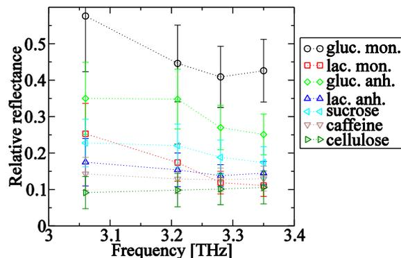
Figure 1. Diffuse reflectance of a range of powdered solids at 3.05, 3.21, 3.28 and 3.35 THz, relative to that of a PTFE reference powder.
