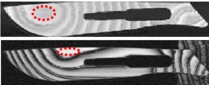
Figure 2: 2.6 THz feedback interferometry images of scalpel blades obtained at ranges of 50 cm (top) and at 10.5 m (bottom). The flat part of the blade used for calculating the figure-of-merit in each image is indicated by a dashed ellipse.
