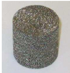
Fig. 1 A cylindrical metal rubber (MR) specimen.
