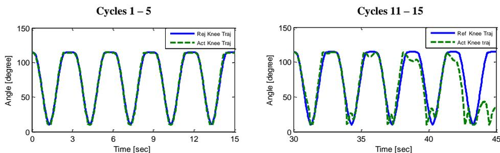
Fig. 8. Knee trajectory with fuzzy logic control
