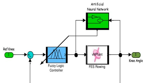
Fig. 2. Block diagram of adaptive neurofuzzy control system
