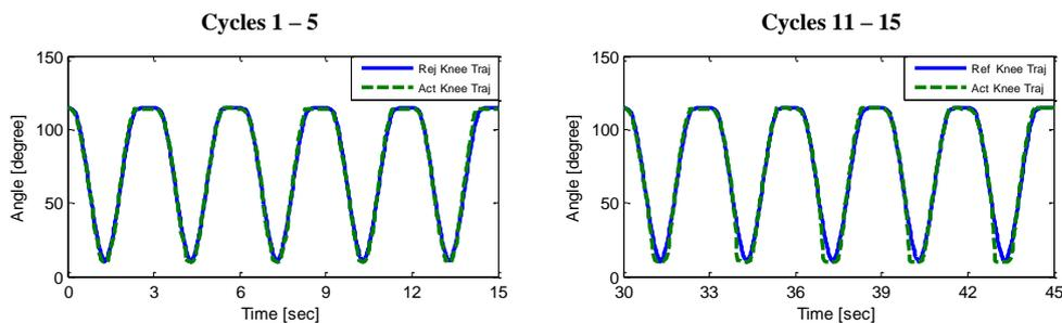
Fig. 9. Knee trajectory with adaptive neurofuzzy controller
