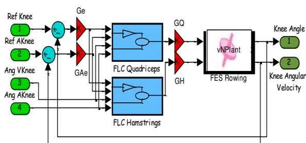
Fig. 5. Block diagram of FLC without adaptation
