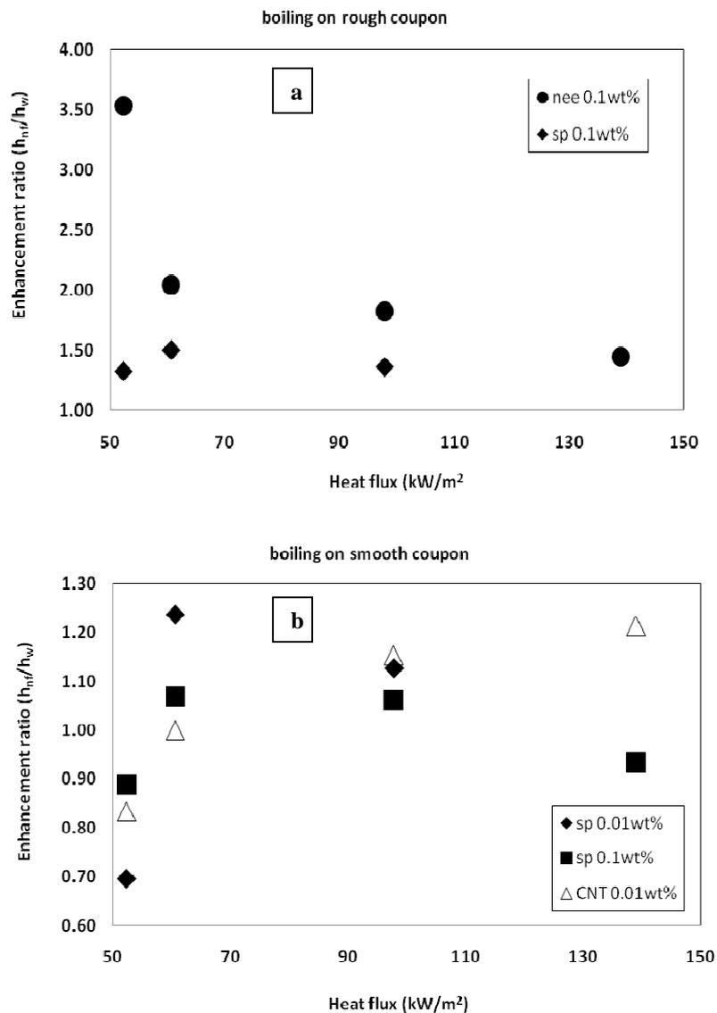
Figure 2: Dependence of heat transfer enhancement on roughness, particle type and shape and concentration
