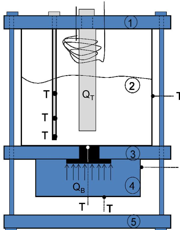
Figure 1: Apparatus; T-thermocouples,  $Q_B$ -heater for copper coupon,  $Q_T$ -auxiliary heater
