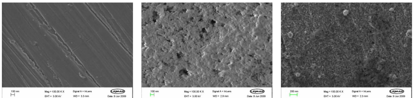
Figure 4: On left, middle & right; A smooth copper coupon, after boiling alumina spheres & alumina needles
