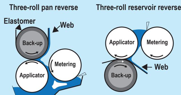
Figure 1 Pan-fed (left) and reservoir-fed deformable roll coating systems
