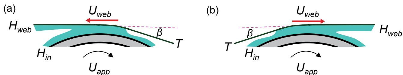
**Figure 5 (a) reverse mode kiss coating nip (b) forward mode kiss coating nip**
