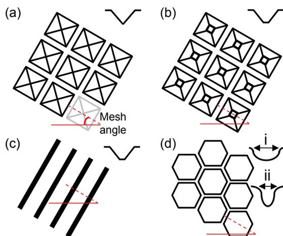
**Figure 2 Schematic showing typical gravure cells. (a) pyramidal, (b) quadrangular, (c) continuous trihelical, (d) laser engraved ceramic cells. A cross-section through each of the cells along the line of engraving is also shown**
