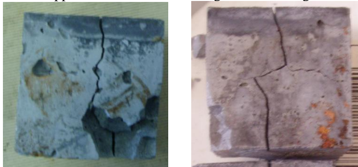
Figure 2 Unsoundness observed in 30%(w/w) APC samples
