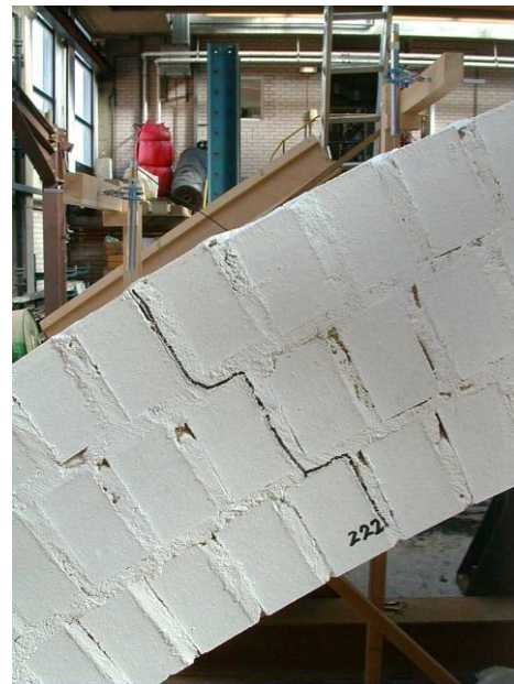
b). 2 nd hinge forming in the arch extrados
