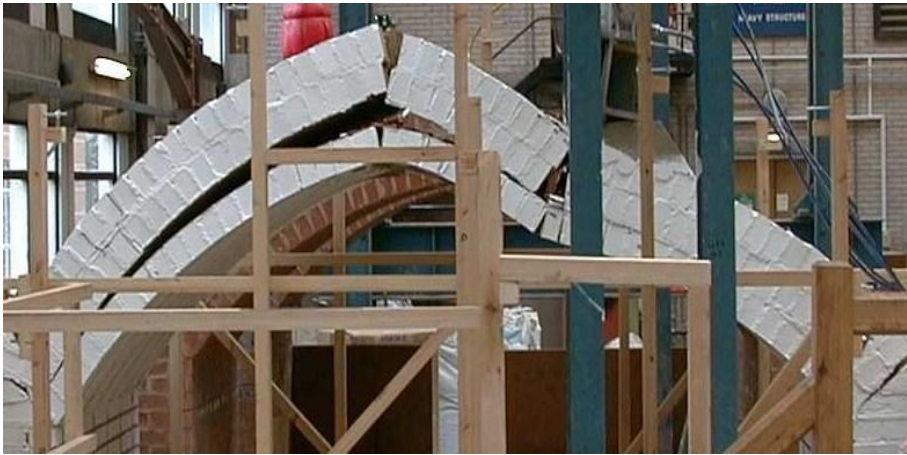
Figure 6. A reinforced arch (arch 2) without shear reinforcement showing premature partial ring separation and a 4-hinge collapse mechanism.
