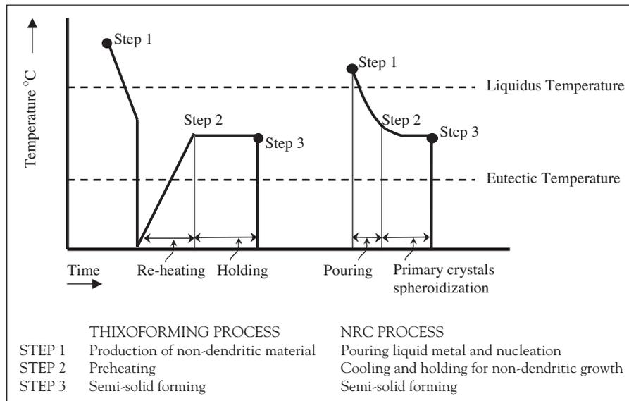
Figure 1: Temperature vs. time for thixoforming and NRC processes.
