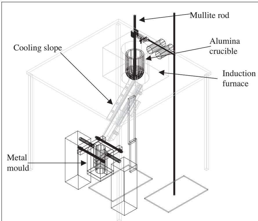
**Figure 3:** Cooling slope with bottom pouring from the crucible.
