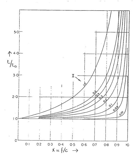
Figure 2. Pollaczek-Khintchine delay curve and deterministic queueing curve
