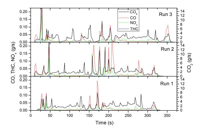
Figure 2: Emissions comparison for the three smooth runs
