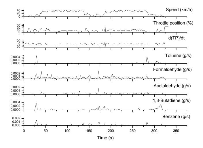
Figure 9: Non-regulated hydrocarbons from smooth run
