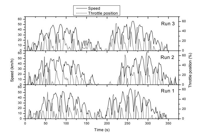
Figure 5: Speed and throttle position for the three speed bump runs
