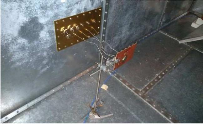
Fig. 2 Measurement Jig in the Reverberation Chamber.
