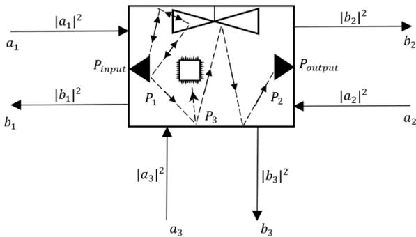
Fig. 5. Power flow in the reverberation chamber.
