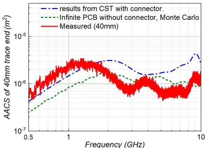
Fig. 12. AACS for 40 mm long track with matched loads
