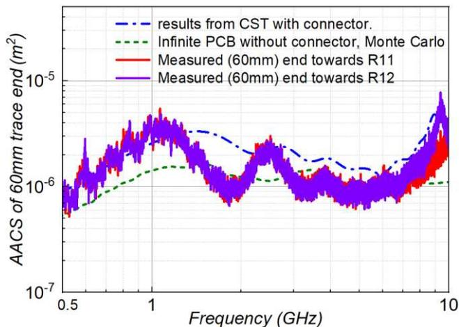
Fig. 11. AACS for 60 mm track with matched loads
