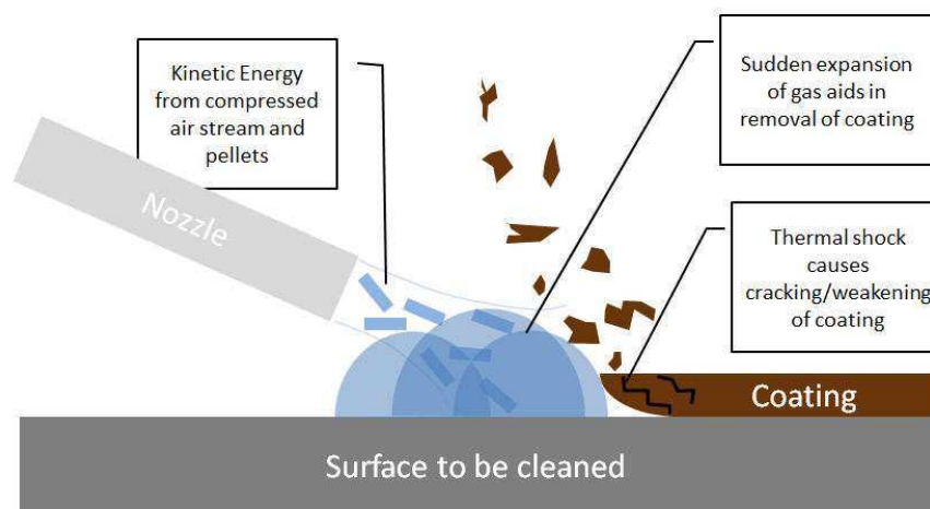
Figure 1. The three mechanisms of dry-ice cleaning
