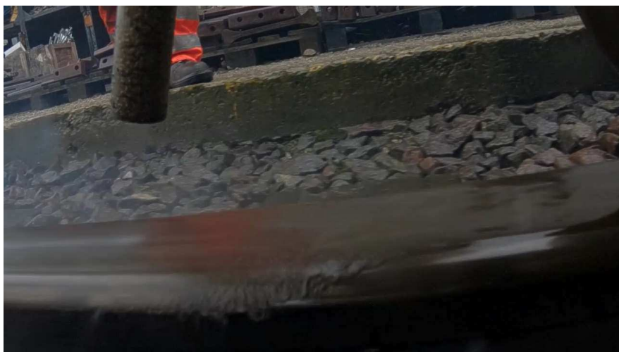
Figure 5. A still from the nozzle camera showing water being removed from the railhead.
