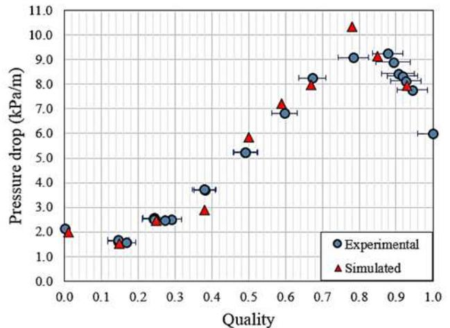
Fig. 2 Comparison between experimental and predicted pressure drop (experimental error on  $\Delta p$  is  $\pm 0.4\%$ ).
