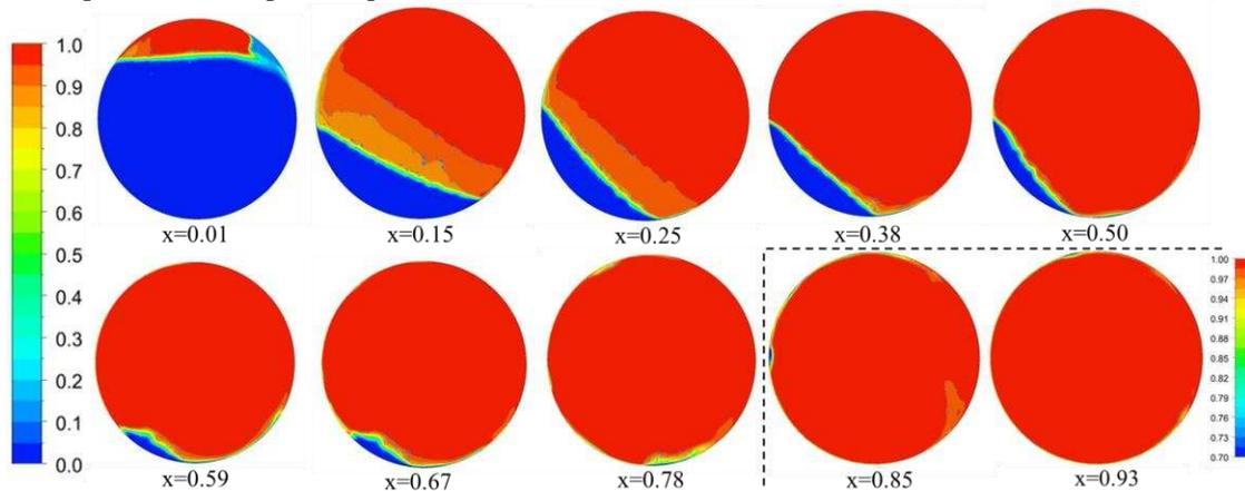
Fig. 3 Void fraction profiles in the tube. The outer part of the coil is at nine o'clock.
