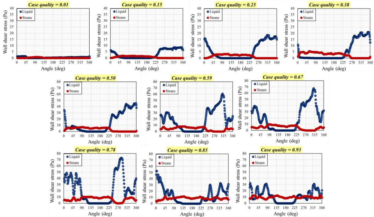
Fig. 4 Wall shear stress profiles:  $0^\circ$  is the outer part of the tube (nine o'clock in Fig. 3) and clockwise convention is used
