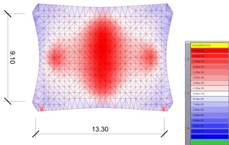
Figure 5: Stress distribution (blue-tension, red-compression)
