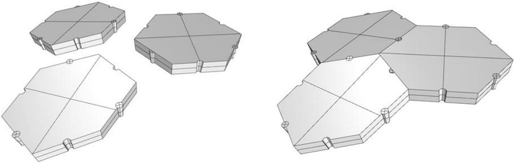
Figure 9: Connection system of the hexagonal panels
