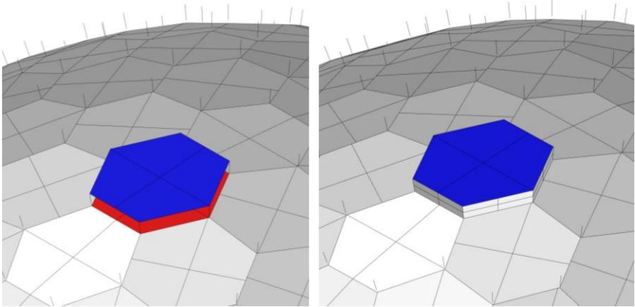
Figure 8: Generation of the extrados (on the left) and contact faces (on the right)
