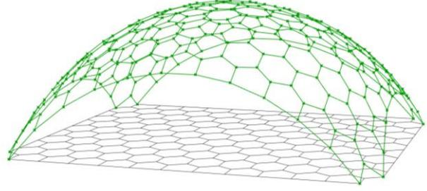
Figure 1: Starting plan with the hexagonal subdivision Figure 2: 3D shape after form-finding before planarization
