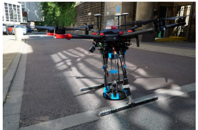
Fig. 2 Asphalt 3D Printing Drone.
