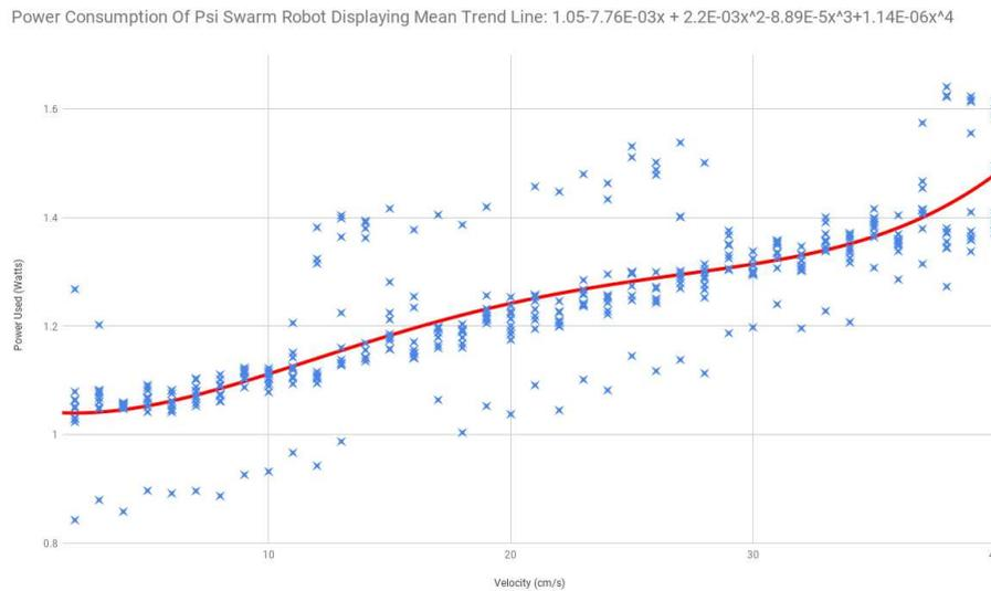
**Figure 2.** Graph displaying the results of the power consumption of a Psi Swarm robot increasing motor speed gradually. 10 repetitions were taken for these results and a trend line has been fit to the mean of these results and is shown in red.
