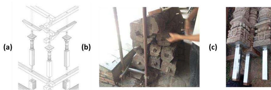
Figure 1: (a) Detail of the connection of the wooden pillars with the rest structural elements (Arce et al. , 2018), (b) typical failure of the vertical timber elements supporting the peripheral walls, and (c) strengthening of timber pins with stainless steel warping (Arce et al. , 2018).
