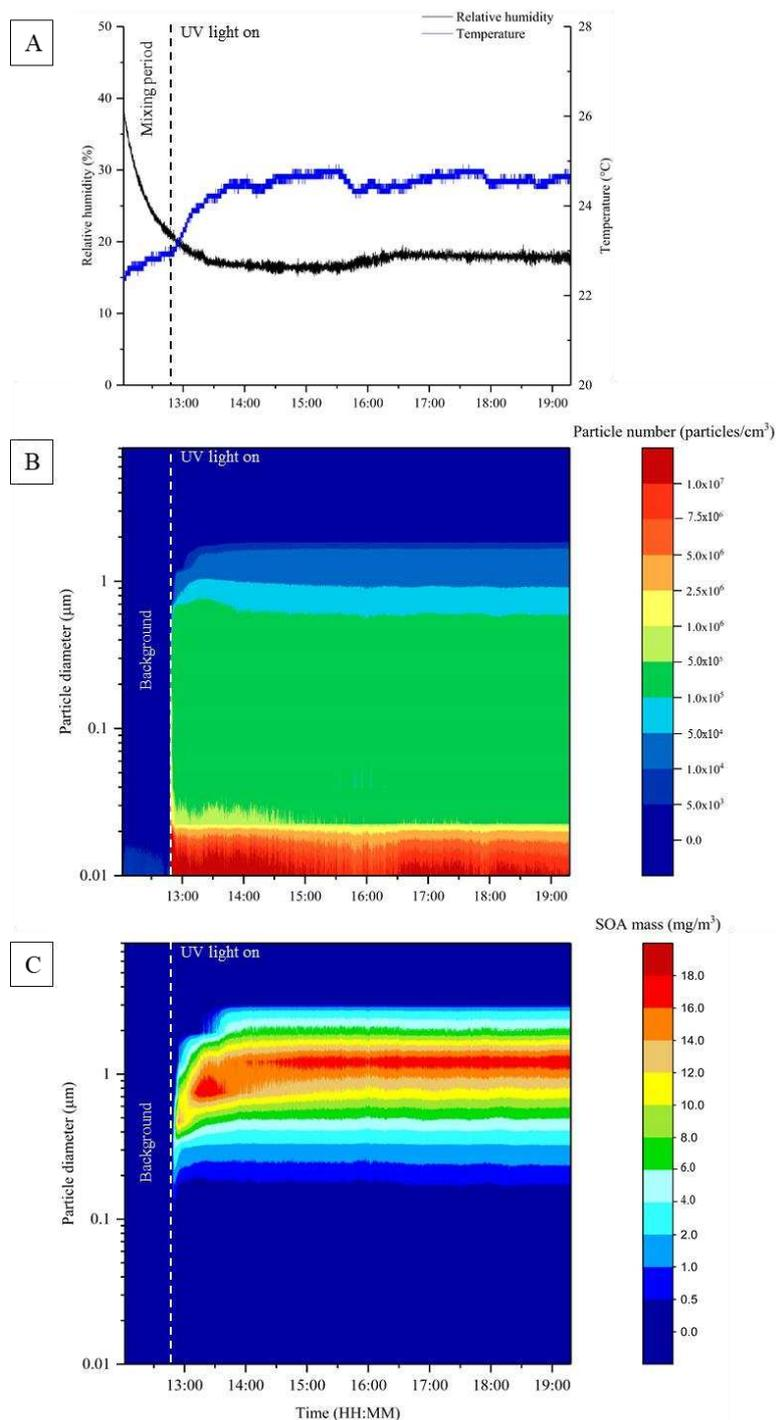
**Figure 2** – Data from a typical CFR experiment, displaying reactor relative humidity and temperature (A), particle diameter and number (B) and particle diameter and mass (C). Measurements are from the photo-oxidation of limonene at 20% relative humidity with a VOC/NO<sub>x</sub> ratio of 13 (exp. 20, Table 1).
