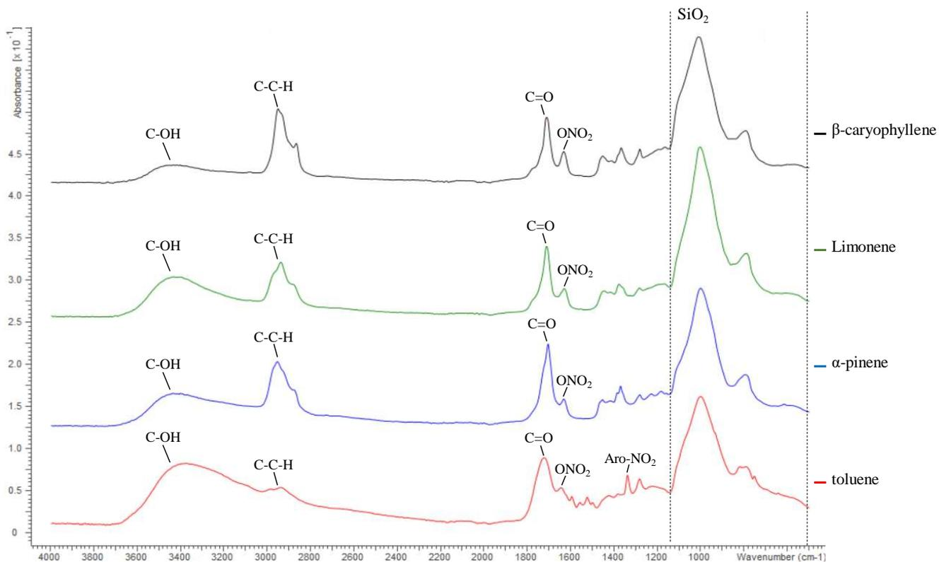
**Figure 4** – ATR-FTIR spectroscopy spectra of  $\beta$ -caryophyllene, limonene,  $\alpha$ -pinene and toluene SOA displaying absorption frequencies of organic functional groups. The quartz filter (i.e. SiO<sub>2</sub>) absorption region is highlighted by a dashed line, see text for further information. Data from experiments 10, 24, 32 and 38, see Table 1. SOA was formed at 55% relative humidity with
