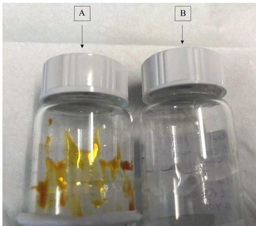
**Figure 3** – Visual differences observed in the light absorbing properties of toluene (A) and  $\beta$ -caryophyllene SOA (B) formed under replicate experimental conditions (55% relative humidity with a VOC/NO<sub>x</sub> ratio of 13, exp. 36 and 31 (see Table 1),
