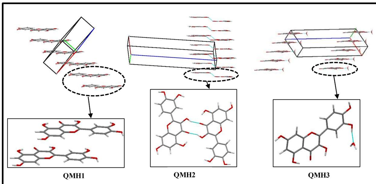
**Figure 7.** Key intermolecular synthons in quercetin monohydrate ordered by synthon strength.
