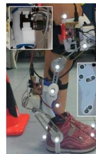
Fig. 9. The details of the WAKE-up system with joint modules and shoe pad [32].
