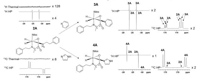
Figure 3. The structure and partial thermal and hyperpolarized <sup>1</sup>H and <sup>13</sup>C spectra for the amine complex 2A are shown. Upon addition of the coligands pyridine or imidazole the complexes 3A and 4A form, the <sup>1</sup>H and <sup>13</sup>C resonances of which hyperpolarize in addition to those of the starting 2A as shown. All <sup>1</sup>H or <sup>13</sup>C spectra are shown on the same vertical scale.
