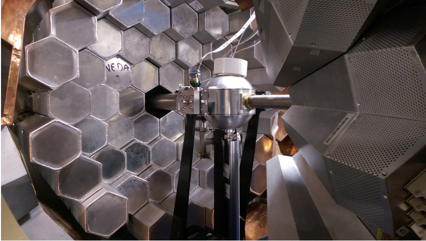
Fig. 2. From right to left (the beam direction): AGATA clusters, ion guide, target chamber with DIAMANT inside, NEDA array. Two triple Neutron Wall detectors are visible in the lower left corner.
