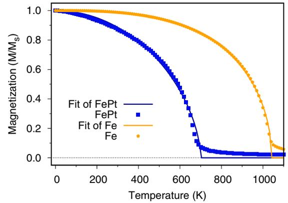
FIG. 1. Calculated temperature-dependent magnetization for Fe and FePt using Monte Carlo simulations. The solid lines represent the fitting using the following expression:  $M(T) = M_0 [1 - (T/T_C)^\alpha]^\beta$ , which gives a Curie temperature of 1050 K for Fe and 700 K for FePt.
