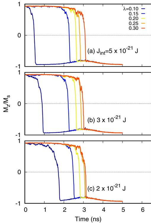
FIG. 4. Calculated evolution of  $z$ -components of reduced magnetization during the reversal mechanism for different interface exchange coupling strength (a)  $J_{\text{int}} = 5 \times 10^{-21}$  J, (b)  $J_{\text{int}} = 3 \times 10^{-21}$  J, and (c)  $J_{\text{int}} = 2 \times 10^{-21}$  J with a variation of damping of the soft layer (Fe). The damping constant of the hard phase (FePt) has been kept fixed at 0.1.
