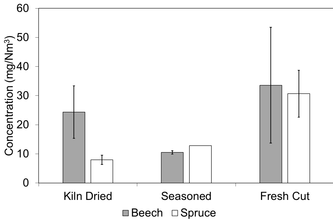
Fig. 4. Total particulate matter results obtained by the Dekati Impactor of the smoke concentrations (mg/Nm 3 ) for refuelled cycles plotted for all fuels studied: ■ beech, □ spruce.
