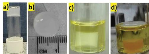
Fig. 2 The preparation of Pd-hybrid hydrogels: (a) inversion test; (b) size of the gel; (c) immersion in PdCl<sub>2</sub> solution; (d) hybrid gel with Pd loaded after 48 hours.
