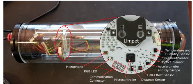
Figure 4: Sensor nodes used in the sea trials
