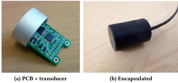
Figure 3: Acoustic “Nanomodem” developed by Newcastle University
