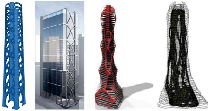
Fig. 1. Structural topology optimisation techniques on buildings [9,10,11].
