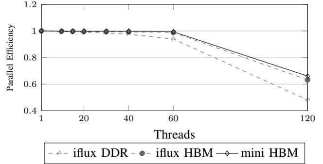
Fig. 7: Parallel efficiency comparison of the mini-app and *iflux* on KNL.
