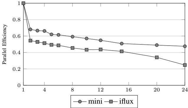
Fig. 4: Parallel efficiency of mini-HYDRA and `iflux`.
