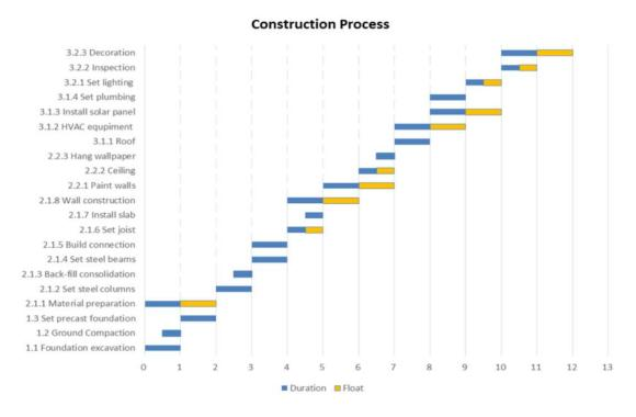
Fig. 13. A demonstration of 12-day on-site construction scheduling
