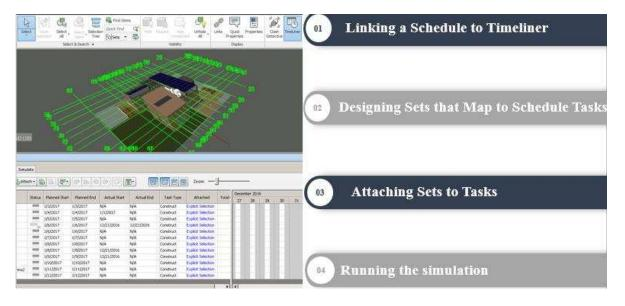
Fig.14. A description of the procedure to simulate 4D scheduling from Microsoft Project to Autodesk Navisworks
