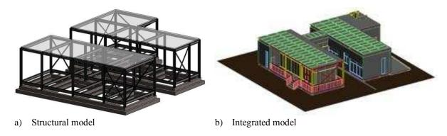
Fig.7. Interdisciplinary collaboration in the structural design
