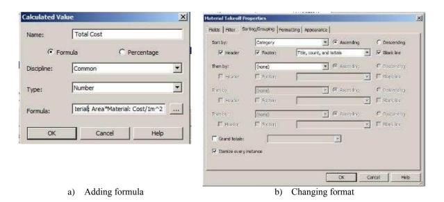
Fig. 16. Students' work on editing existing quantity take-off functions in Autodesk Revit
