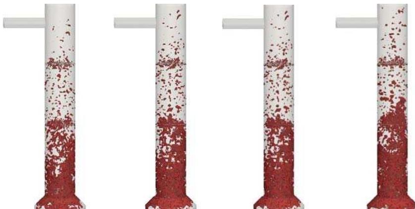
Fig. 8. Iso-surface of  $\alpha$  Showing the Isolated Dispersed Phase Fluid at times 0 s, 0.25 s, 0.5 s, and 0.75s from Left to Right Respectively.
