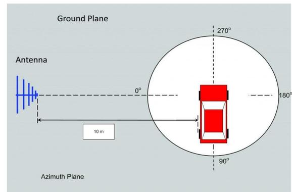
Fig. 1. CISPR 12 Radiated Emissions Measurement Configuration
