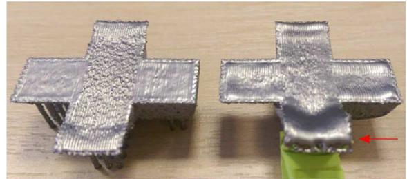
Fig. 9. Physical cross pieces showing evidence of swelling (indicated with marker).
