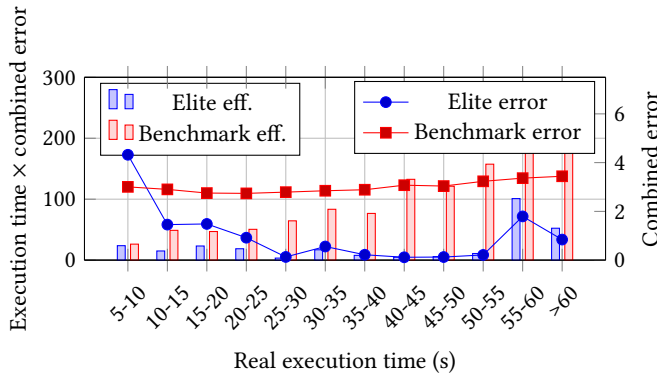
Figure 8: Average run time × combined error for each algorithm, using as many generations as possible in time limit, optimal parameters for each algorithm and population of 50.
