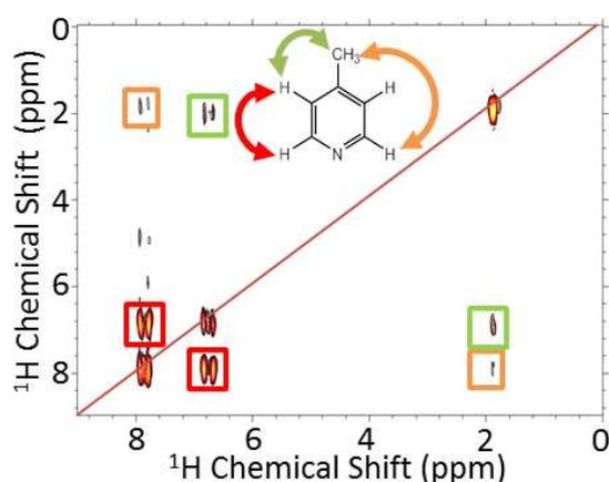
Figure 6 2D gradient selective COSY coupled with SABRE for 52 mM 4-methylpyridine and 5.2 mM catalyst in methanol-*d*<sub>4</sub>. The COSY measurements used 64 increments over a bandwidth of 500 Hz (11.5 ppm), with single scan transients and re-hyperpolarization between each point. The total experiment time was around 36.4 minutes.
