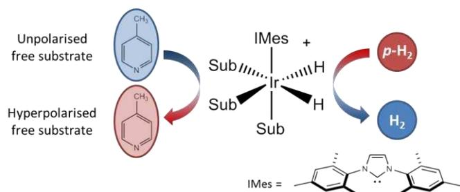
Figure 1 An active SABRE catalyst reversibly binds both  $p\text{-H}_2$  and a substrate to allow polarization transfer from  $p\text{-H}_2$  to the substrate in a polarization transfer field (PTF) of a few tens of gauss.
