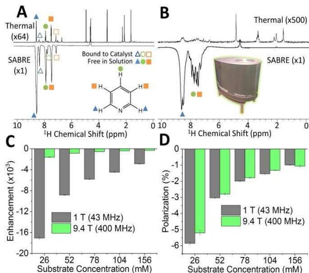
Figure 2 Comparison of thermally polarized (top) and SABRE hyperpolarized (bottom)  $^1\text{H}$  NMR spectra of 52 mM pyridine with 5.2 mM catalyst in methanol- $d_4$  for NMR detection at (A) 9.4 T and (B) 1 T. (C) SABRE enhancement factor,  $\epsilon$ , and (D) polarization level,  $P$ , for the *ortho* resonance (blue triangle) as a function of substrate concentration with NMR detection at 1 T (gray) and 9.4 T (green). Error bars represent the standard deviation across 5 measurements.
