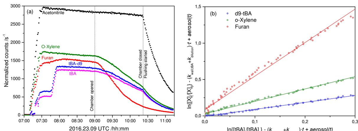
**Figure 4.** (a) Time evolution of tBA, d<sub>9</sub>-tBA, the reference compounds o-xylene and furan, and the inert dilution tracer acetonitrile as observed during a relative rate experiment in the EUPHORE chamber. (b) Double-logarithmic plot showing the OH-induced decay of furan (black), o-xylene (red) and d<sub>9</sub>-tBA (blue), respectively, relative to the decay of tBA. The data have been corrected for dilution losses and partitioning to the chamber walls and particles formed.
