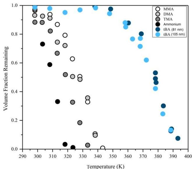
**Figure 7. Thermal properties comparison of tB-aminium nitrate with corresponding nitrates from monomethylamine (MMA), dimethylamine (DMA) and trimethylamine (TMA). Data for ammonium nitrate have been included for reference. Two separate experiments with initial particle diameters of 81 and 105 nm, respectively, were carried out with tB-aminium nitrate particles.**
