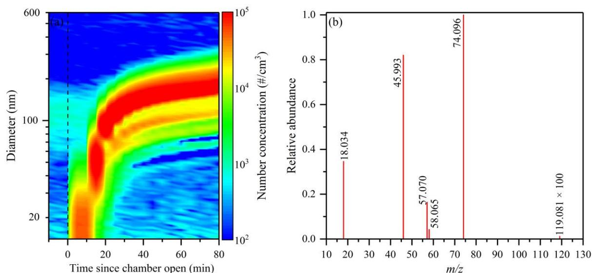
**Figure 6. (a) Particle size distribution in the EUPHORE chamber as function of time (b) CHARON-PTR-ToF-MS mass spectrum obtained from the particles formed when tBA was reacted with OH radicals in the presence of  $\text{NO}_x$ .**
