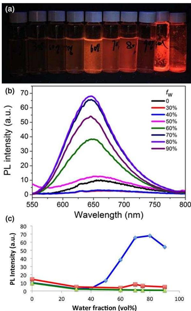
**Figure 4.** (a) Photograph of **7a**  $10^{-5}$  M in THF-water mixtures with different vol% values (from left to right ( $f_w$ ): 0 %, 30 %, 40 %, 50 %, 60 %, 70 %, 80 %, 90 % and solid) taken under UV illumination at 365 nm; (b) Emission spectra of **7a** in THF-water mixtures,  $\lambda_{ex} = 530$  nm; (c) Change in PL intensity of **7a** (blue), **7b** (red) and parent complex  $[\text{Ir}(\text{ppy})_2(\text{deeb})][\text{PF}_6]$  (green).
