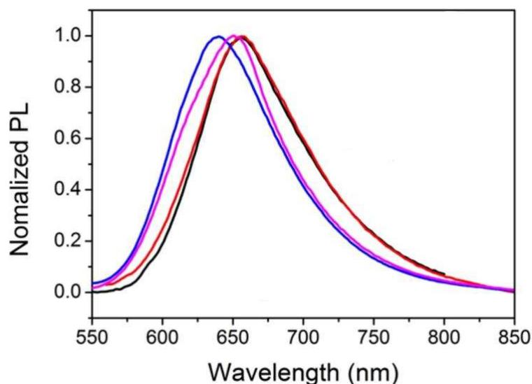
**Figure 3.** Emission spectra ( $10^{-5}$  M) of **7a** (black: in  $\text{CH}_2\text{Cl}_2$ ; blue: neat film) and **7b** (red: in  $\text{CH}_2\text{Cl}_2$ ; mauve: neat film).
