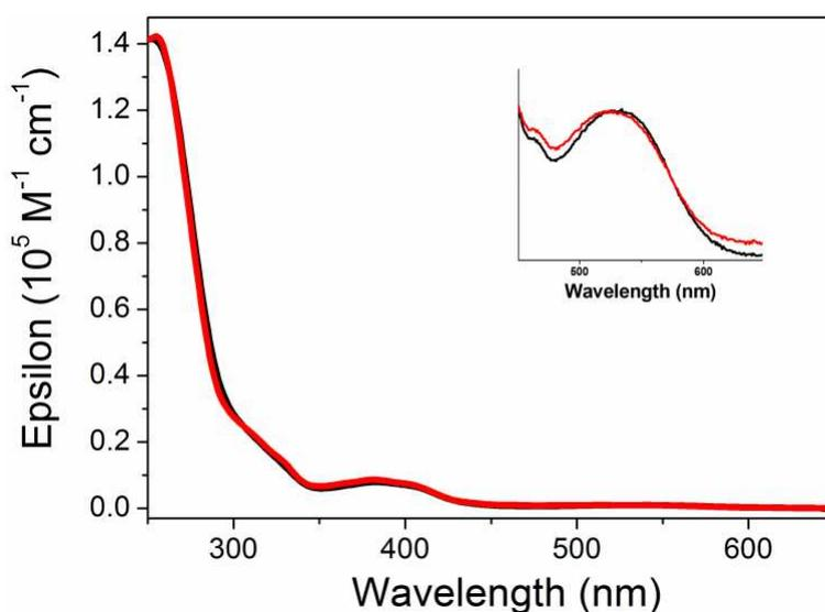
**Figure 2.** UV-vis spectra of **7a** (black) and **7b** (red) in CH<sub>2</sub>Cl<sub>2</sub> at room temperature (10<sup>-5</sup> M). Inset: zoom into the 500-600 nm region (10<sup>-4</sup> M).
