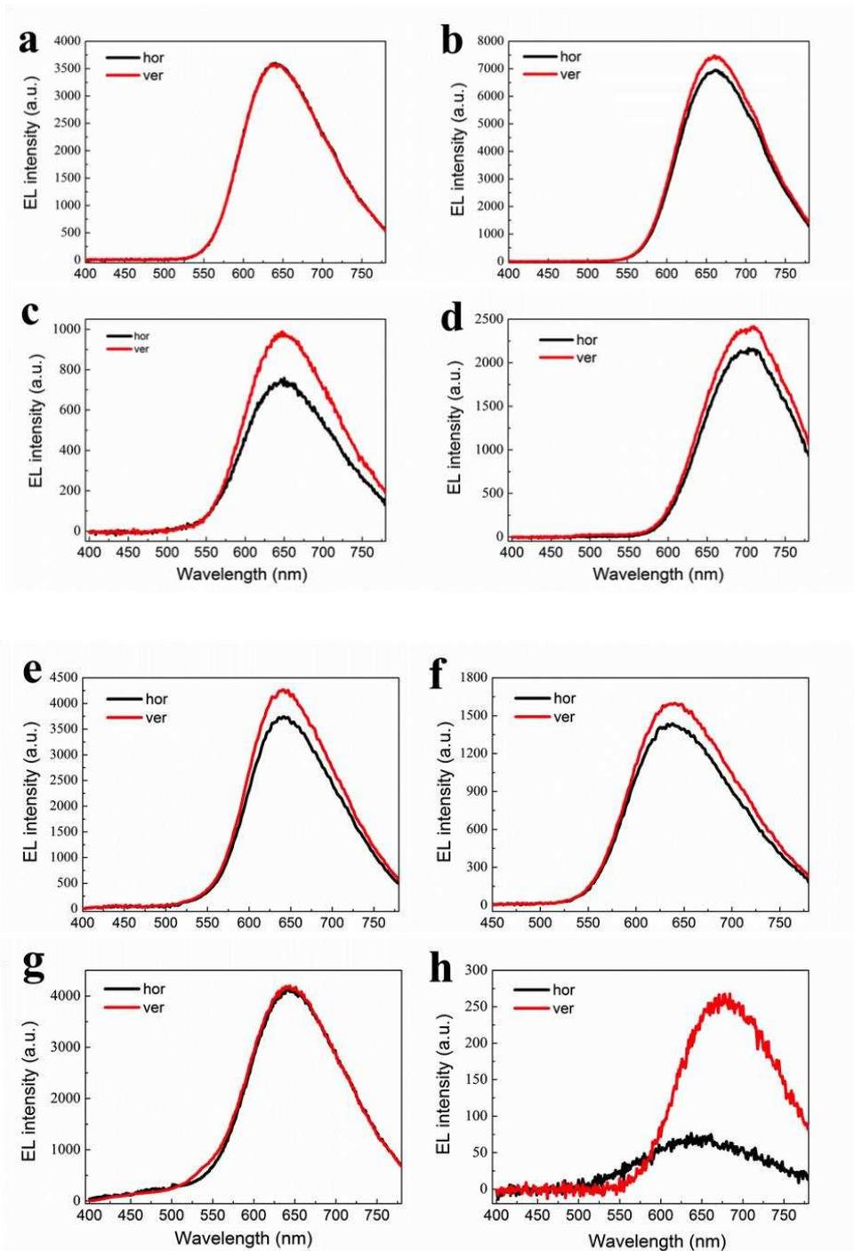
**Figure 5** EL spectra from devices I, II, III and IV at 10 mA/cm<sup>2</sup> after a linear polarizer at two orthogonal directions (vertical: parallel to rubbing direction; horizontal: orthogonal to rubbing direction): (a) **7a** in device I; (b) **7a** in device II; (c) **7b** in device I; (d) **7b** in device II; (e) **7a** in device III; (f) **7a** in device IV; (g) **7b** in device III; (h) **7b** in device IV.
