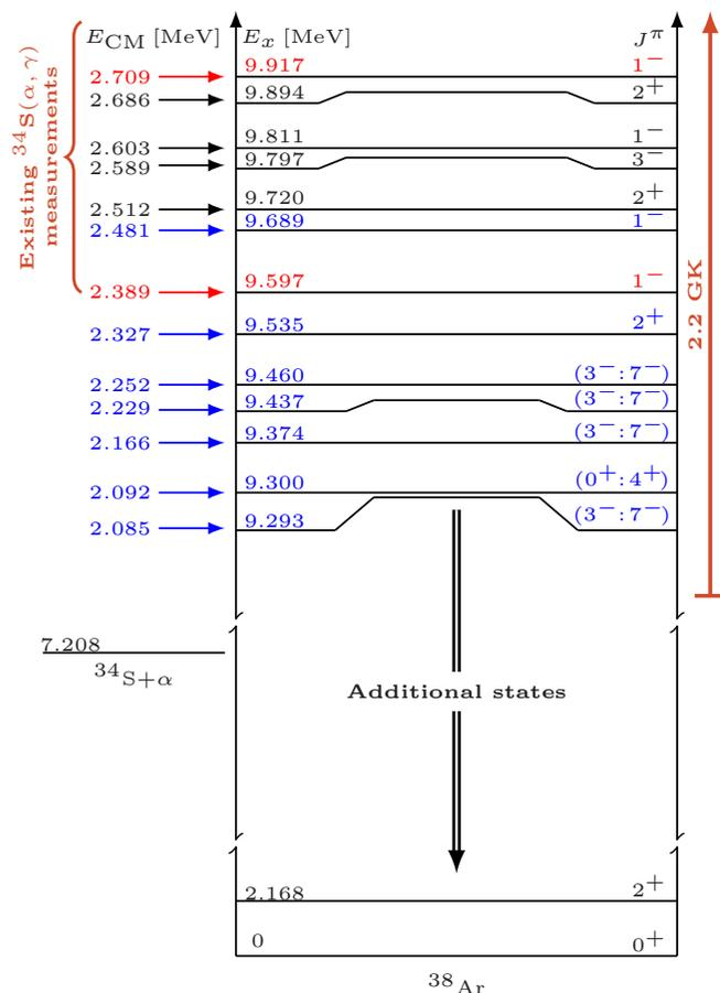
FIG. 1. Partial level diagram of  $^{38}\text{Ar}$ . States in blue were measured in this work. The two states in red (also measured in this work) are those for which there exists broad uncertainty in the literature values for the resonance strengths. Excitation energies are those reported in Ref. [16]. The astrophysically relevant energy range for oxygen burning (calculated from Ref. [7]) is illustrated on the right.
