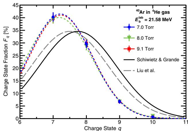
FIG. 7. CSD measurements of  $^{40}\text{Ar}$  passing through  $^4\text{He}$  gas at a laboratory-frame bombarding energy of  $E_b^{\text{lab}} = 21.58$  MeV. The black and dashed gray curves are the average equilibrium CSDs predicted by the semi-empirical formulas of Refs. [35,36], respectively.
