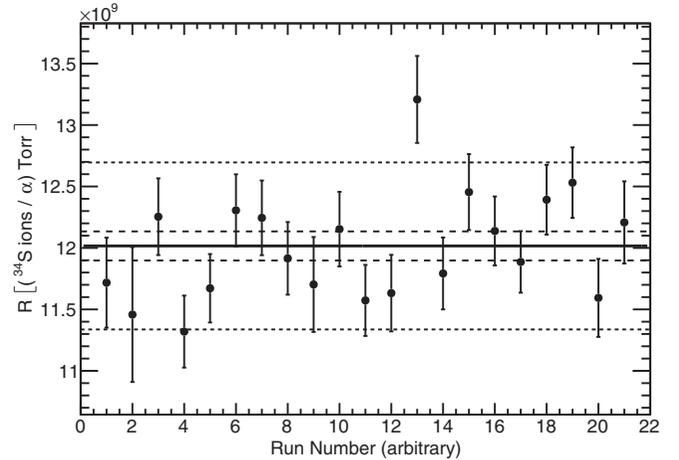
FIG. 5. Beam normalization coefficients  $R$  for all runs during the yield measurement of the  $E_{\text{CM}} = 2166$  keV resonance. The solid horizontal line is the value of  $\bar{R}$  obtained from a  $\chi^2$  fit to the data. Dashed horizontal lines are the statistical uncertainty in  $\bar{R}$ , and dotted horizontal lines are the total (statistical and systematic added in quadrature) uncertainty in  $\bar{R}$ .
