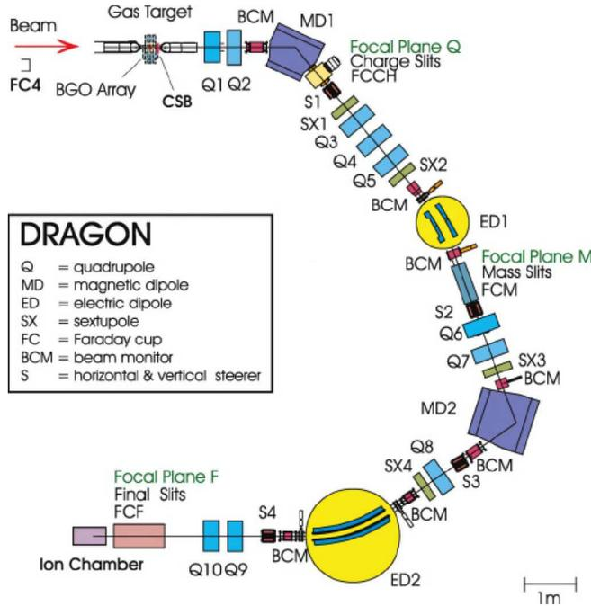
FIG. 2. Schematic of the DRAGON recoil mass separator.
