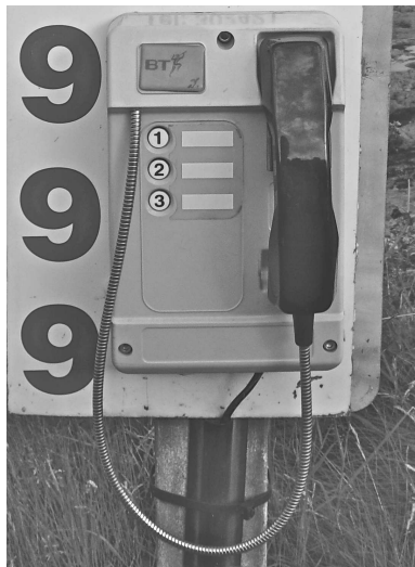
Figure 1: A very simple walk-up-and-use user interface. A UK Coast Guard phone (photographed in 2016) for the public to use to call the Coast Guard in the event of an emergency. In the UK, the standard emergency number is 999 — as the sign makes very clear. But the phone itself does not have any way to dial 999, so what should you do? It is not very clear! Presumably only three buttons (labelled 1, 2, 3) were provided either to make it “simpler” or to save money? Figure 2 shows the underlying FSM for this phone, and the FSM shows how to use the phone to correctly call the Coast Guard.
