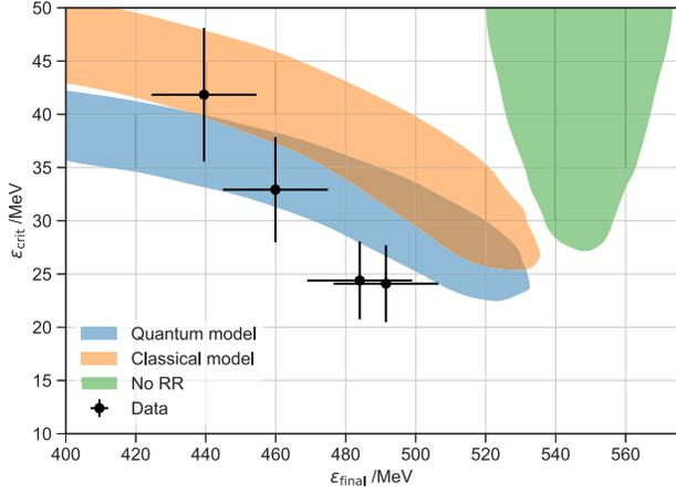
FIG. 9. Experimentally measured  $\epsilon_{\text{crit}}$  as a function of  $\epsilon_{\text{final}}$  measured at the electron spectral feature (points). The shaded areas correspond to the results a hypothetical ensemble of identical experiments would measure 68% of the time under different assumed radiation reaction models for a uniform distribution of  $a_0$  between 4 and 20.
