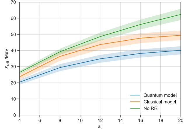
FIG. 8. Simulated retrievals of  $\epsilon_{\text{crit}}$  assuming the collision of a plane wave of given peak  $a_0$  with the experimentally measured electron spectra. The shaded regions represent  $\pm 1\sigma$  variations arising from the measured electron beam spectral fluctuations.
