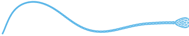
Figure 3: The tapering flagellum used for the power calculations, where in contrast to velocity field and trajectory calculations, which are insensitive to such details, the flagellum profile has a non-trivial, but modest, influence on the modelling predictions.
