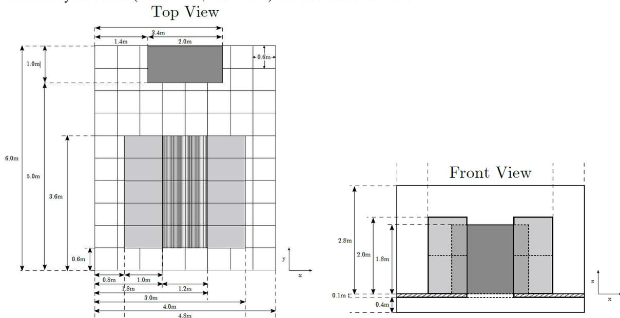
Figure 6 – Plan and front view with dimensions of the benchmark case study data center
