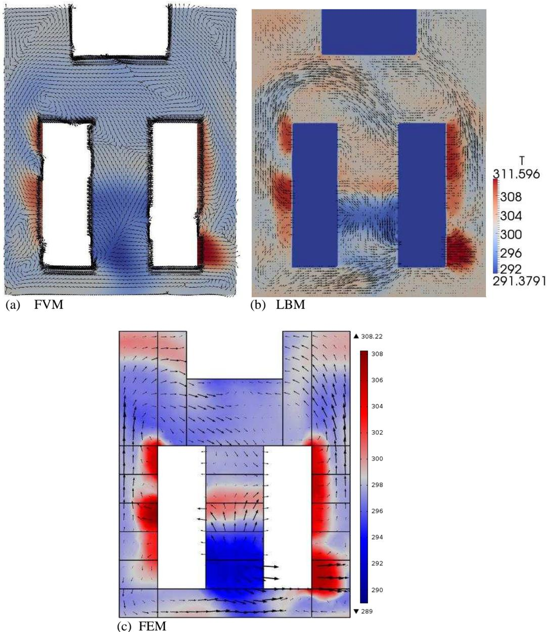
Figure 14 – Cross section horizontal plane at 1.5m from the data center floor,  $z = 1.5$ . Results show temperature and air velocity for (a) FVM, (b) LBM and (c) FEM. Temperature scales are in Kelvin.
