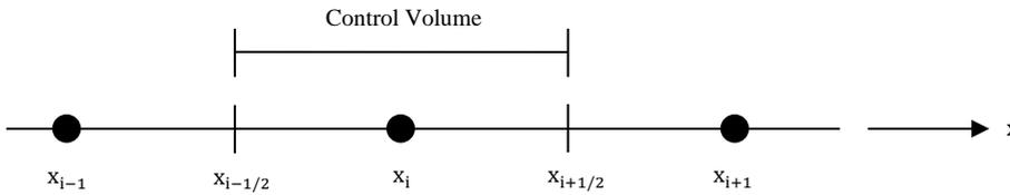
Figure 3 – Sketch of a control volume for the finite volume discretisation of the x-dimension
