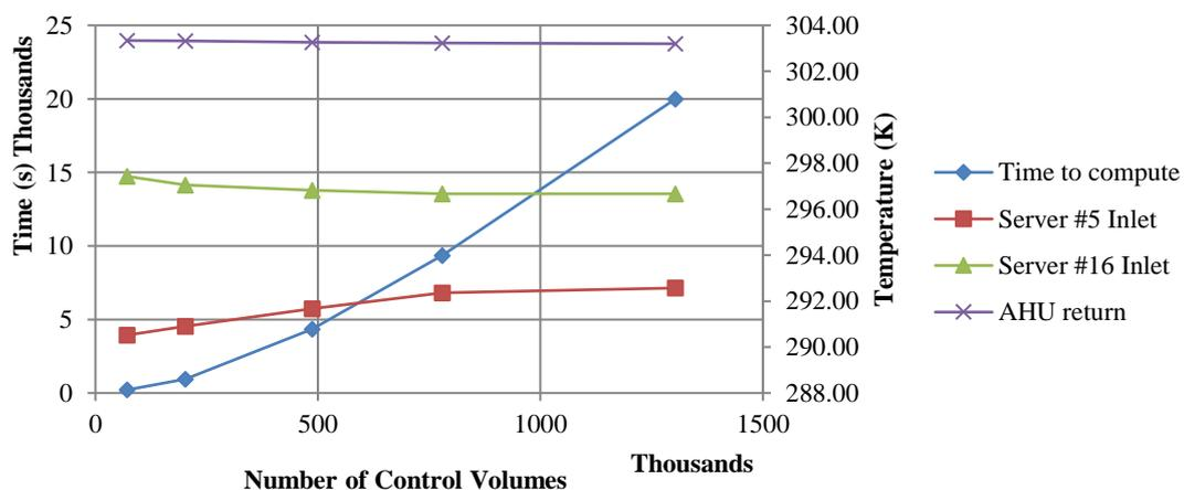
Figure 9 – FVM mesh refinement on the calculated boundary temperatures at certain points in the data center.
