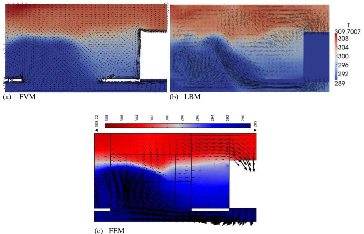
Figure 13 – Cross section plane down the middle of the cold aisle at  $2.4\text{m}$  from the side of the data center,  $x=2.4$ . Results show temperature and air velocity for (a) FVM, (b) LBM and (c) FEM. Temperature scales are in Kelvin.
