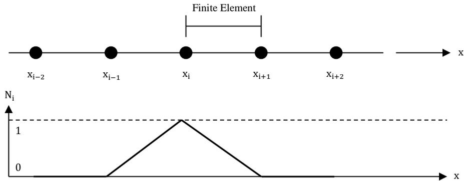
Figure 1 – Sketch of linear finite elements along the x-dimension
