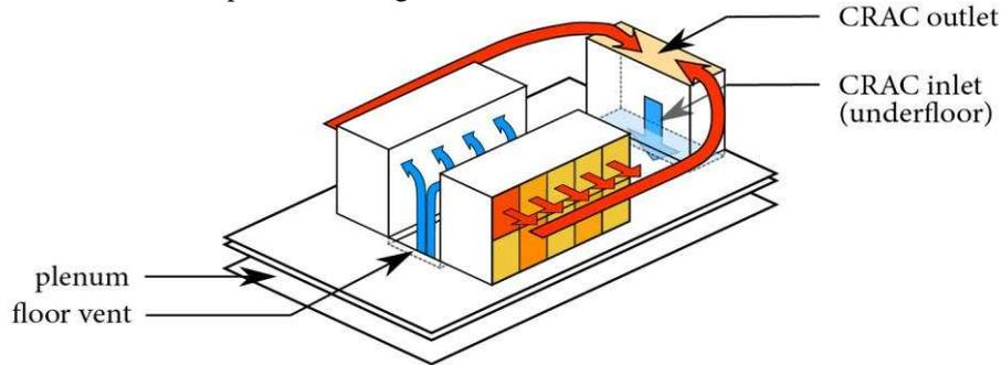
Figure 5 – Schematic of the benchmark case study data center in cooling operation. Temperatures and airflows indicated by the colour (warm – red; cool - blue) and direction of the arrows.
