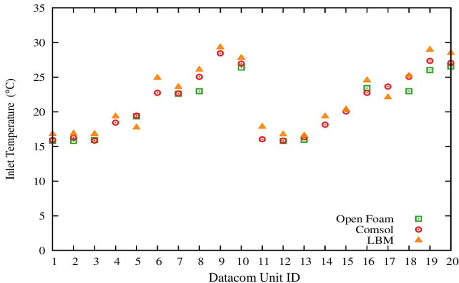
Figure 15 – Inlet temperatures of datacom equipment based on their position in the data center (for the ID refer to Figure 7) as calculated from the three computational methods.
