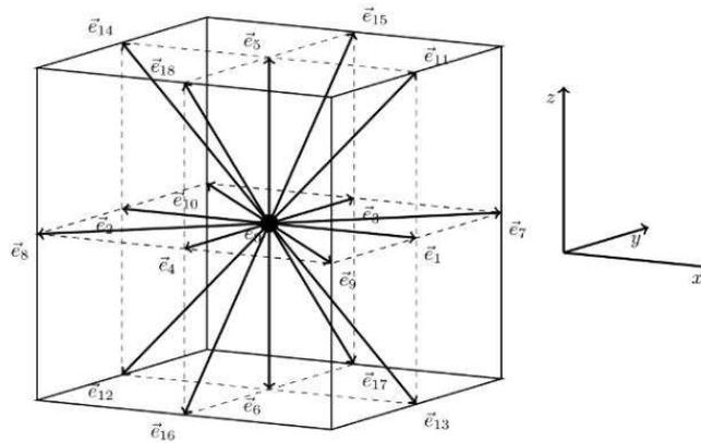
Figure 4 – Discretisation of the microscopic velocities in 3D (D3Q19), which is a nineteen velocity (three speed) lattice.
