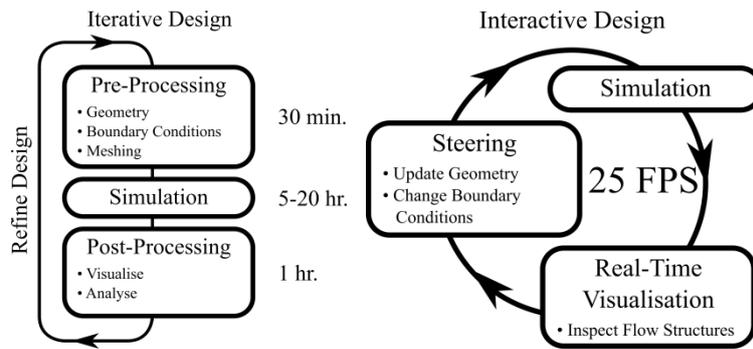
Figure 10 – Contrasting the solution procedures of traditional CFD on the left (FEM and FVM) with real-time CFD on the right (LBM).
