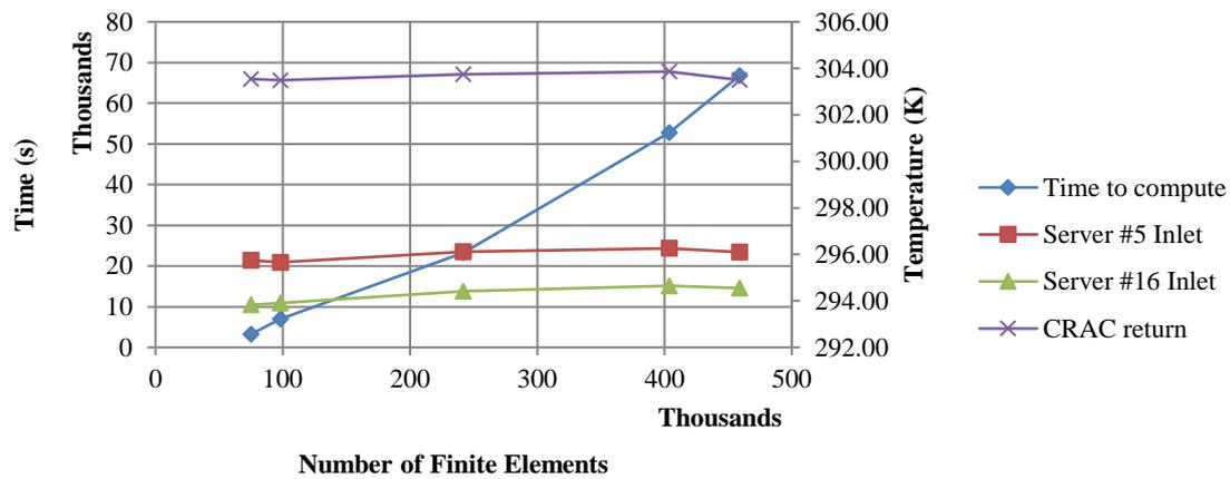
Figure 8 – Mesh refinement on the calculated boundary temperatures at certain points in the data center based on the FEM.
