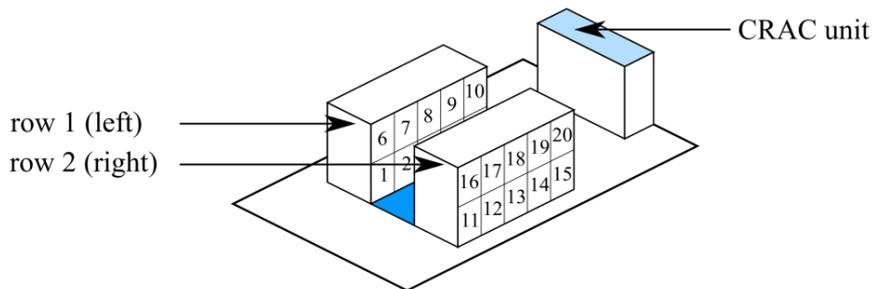
Figure 7 – Layout of datacom units as half rack units.
