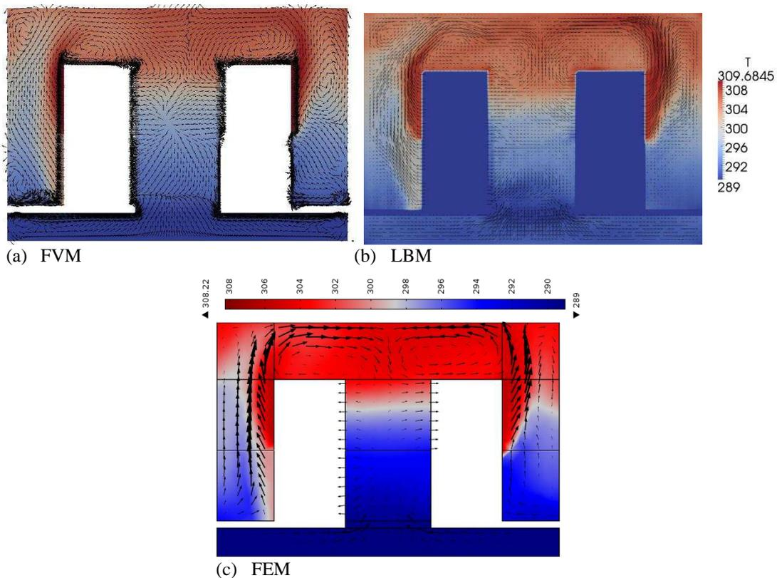
Figure 12 – Cross section plane through hot and cold aisles at 3.4m from the end of the data center,  $y = 3.4$ . Results show temperature and air velocity for (a) FVM, (b) LBM and (c) FEM. Temperature scales are in Kelvin
