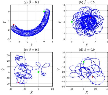
**Fig. 3.** Trajectories  $\mathbf{X}(\tau)$  of the ball centre for  $\mu = 1$ ,  $\gamma = 1$ ,  $\rho = 1/2$ ,  $\tilde{\beta}$  as shown, and  $\tilde{\delta}$  given by [40]; initial conditions [41] and [42]. Lyapunov exponents: (a)  $\lambda \approx 0.002$ ; (b)  $\lambda \approx 0.003$ ; (c)  $\lambda \approx 0.053$ ; (d)  $\lambda \approx 0.077$ .
