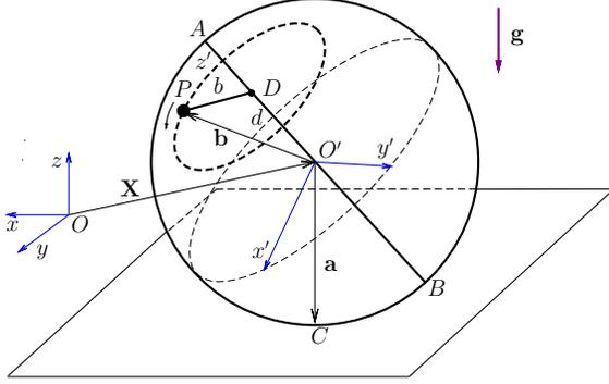
**Fig. 1.** Configuration sketch: the spherical shell rolls on a horizontal plane; the rod  $AB$  is on bearings at  $A$  and  $B$  that allow it to rotate freely about its axis; the rod  $DP$  is rigidly fixed at  $D$  at right angles to  $AB$ ; a point mass  $m$  is fixed at  $P$ , and the rod structure  $APB$  is driven by a battery mechanism to rotate about  $AB$  with constant angular velocity  $\sigma$ ; the axes  $O'x'y'z'$  are fixed in the spherical shell.
