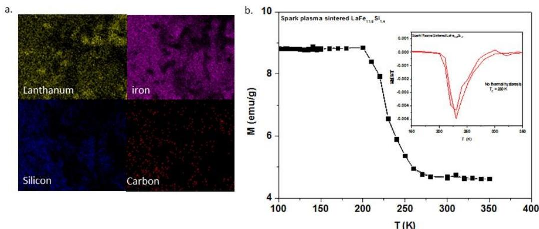
**Figure 2a.** EDS elemental mapping of the La(Fe,Si)<sub>13</sub> sample 6. **2b.** Magnetisation as a function of temperature of sample 6  $\mu_0H = 0.02$  T. **Inset:**  $dM/dT$  of La(Fe,Si)<sub>13</sub> sample 6.
