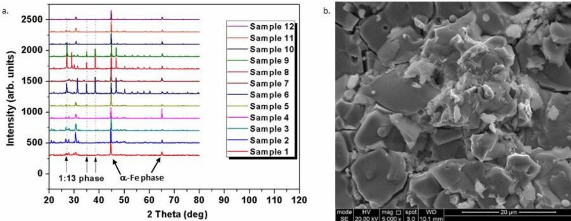
**Figure 1a.** XRD of the different SPS La(Fe,Si)<sub>13</sub> alloys. **1b.** Backscattered SEM micrograph of La(Fe,Si)<sub>13</sub> sample 6.
