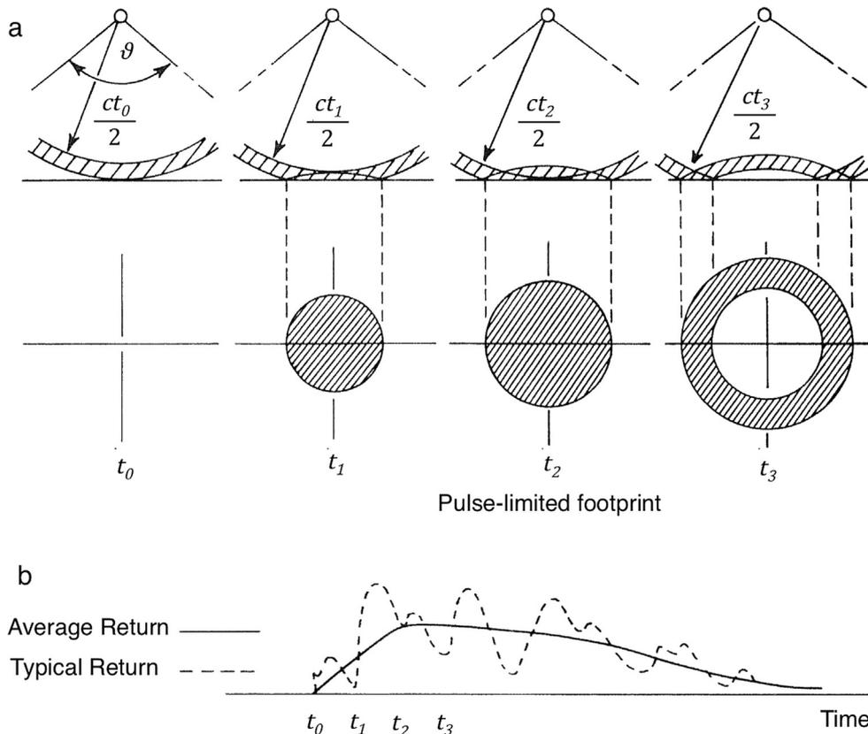
Fig. 6. Development of the illuminated surface area and return waveform for a pulse-limited altimeter. (a) Illuminated surface area for an antenna with beam width  $\theta$ , at times  $t_0$ - $t_3$ . (b) The average return waveform and a typical individual return. Adapted from Rapley et al. (1983).
