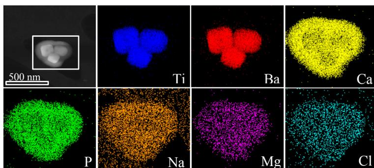
**Figure 2:** STEM-EDX data of DC BT in CCCM. In the EDX spectrum Ca and P are the most prominent peaks but also present were Cl, Mg and Na, all of which spatially match to the coating imaged around the BT nanoparticles.
