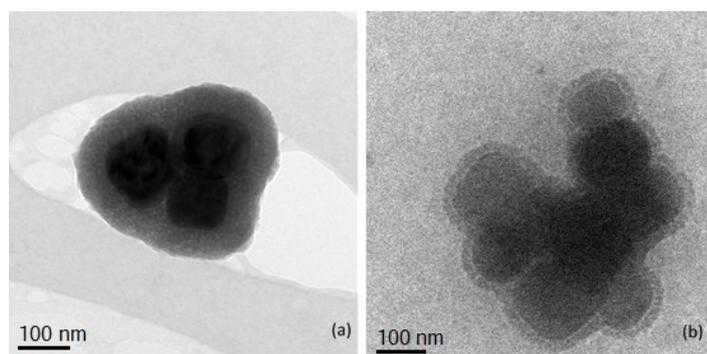
**Figure 1:** (a) TEM image of DC BT in CCCM showing a coating had formed around the nanoparticle agglomerates. (b) This was confirmed in cryo-TEM imaging where a similar coating was observed.
