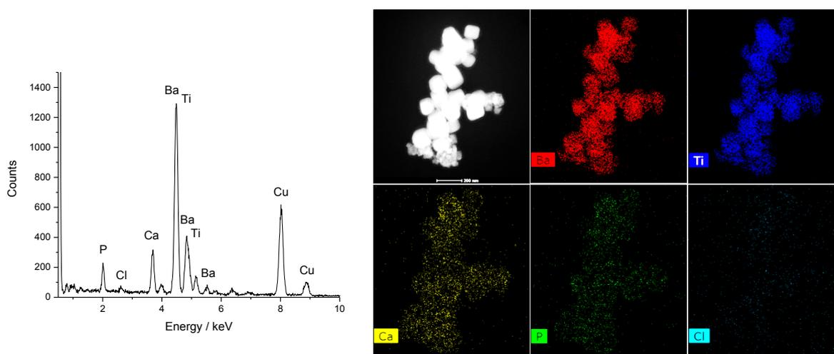
**Figure 3:** Cryo-EDX spectrum and corresponding EDX maps for BT dispersed in CCCM. Ca and P are present in the spectrum but through cryo analysis no visible Na and Mg peaks were present and the Cl peak was only just distinguishable. Analysis was carried out using a probe current of 40 pA.
