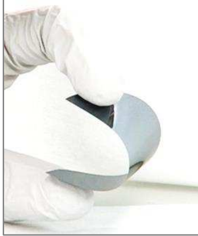
FIG. 1. Crystalline silicon wafers become flexible at ca. 70\ \mu\text{m} thickness. Accordingly, they can be bent to be used for screening the inner surface of a 2" diameter pipe for alpha-contamination and can be mounted on an elastic inspection gauge.
