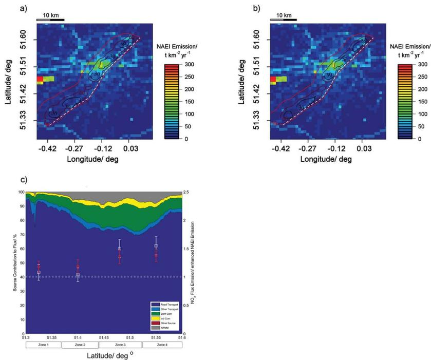
Fig. 3 a) The original footprint calculated using the Drew *et al.* roughness length as in our paper, b) the footprint calculated when we double the roughness length and c) the effect of this on the measured/NAEI emission ratio (white points are the original data, red points are the new data)
